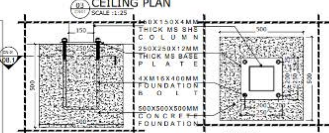
CANOPY-1 DETAIL SCALE: 1:18
