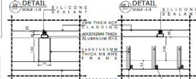
CANOPY-1 DETAIL SCALE: 1:15
